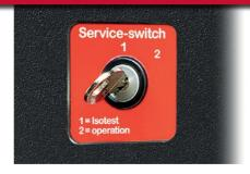
This key switch disconnects all electronic components from the tested load circuits that would cause incorrect readings during an insulation test.
